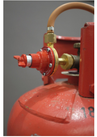
2) Connect gas regulator to gas cylinder, and open valve.
