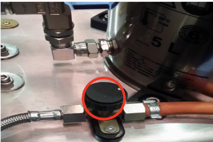
3) Slowly open Gas Valve sufficient to just hear the hissing of the gas
