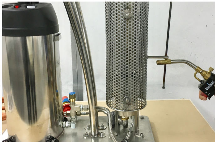
4) Ignite gas with a benzo, and allow coil to heat up to a dull red.
