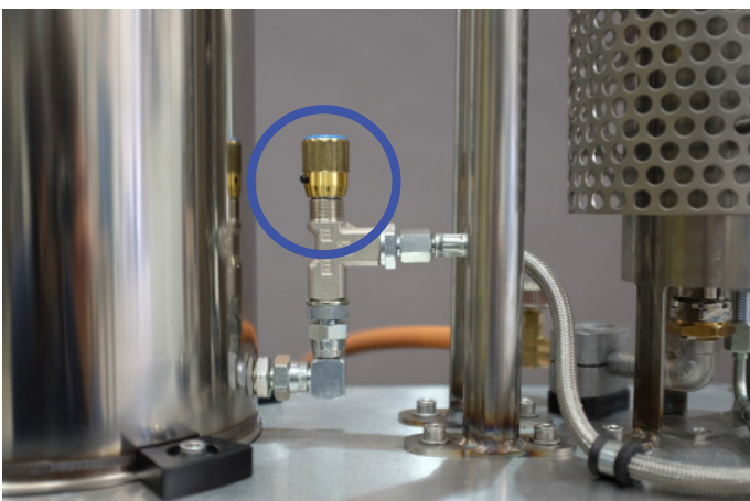
5) Adjust smoke output knob accordingly
