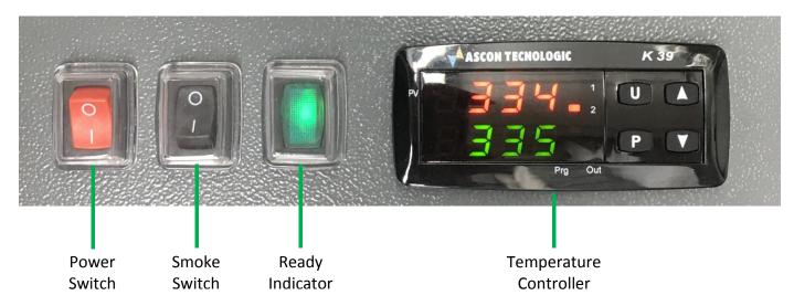
**Temperature Controller:** The temperature controller displays two temperatures. In **RED**, on top is the current heat exchanger temperature. In **GREEN**, on the bottom is the target temperature.
